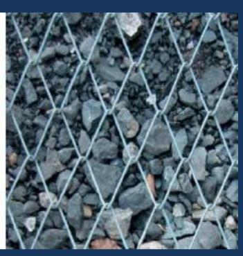
Geobrugg Mesh – is a Ø3mm steel wire, single twisted into meshes in the shape of rhomboids (Diamonds) that offer a great deal of flexibility in all directions.
