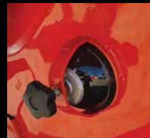
Sight glass for water level indication
