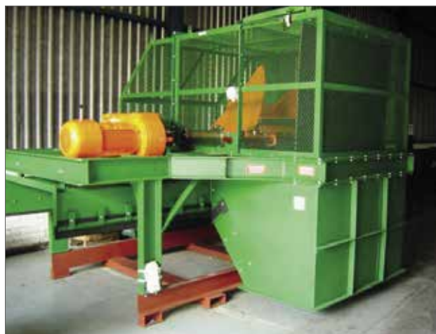
Cross Belt Sampler with Angled Cutter
