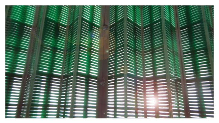
Multotec TeePee™ panels are injection moulded, ensuring repeatable class-leading performance. Computer controlled injection machines maintain optimum conditions throughout the manufacturing process, resulting in consistent aperture sizing in a robust and hard wearing polyurethane.
