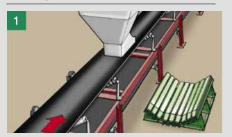
Place the Multotec Loading Point next to the conveyor, with the tapered leading end facing the tail end of the conveyor. Make sure the conveyor is locked out according to your company procedures.
