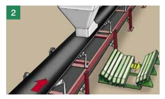
Unbolt the one side of the Multotec Loading Point and remove it from the bottom section of the frame.
