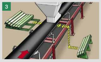
Insert the Multotec Loading Point underneath the conveyor belt. When the Multotec Loading Point is in position, reattach the unbolted side section.
