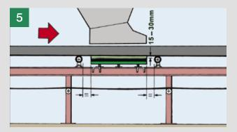
The correct clearance between the underside of the conveyor belt and the Multotec low friction bars is essential. When the conveyor is empty and fully tensioned, there must be a clearance of between 15 to 30 mm. This will depend on the belt dimensions. This is to allow the low friction bars to cool down when the belt runs empty and between loading peaks.
