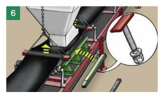
Worn low friction bars are easily replaced. Lock out the conveyor according to your company procedures. Lift the conveyor belt slightly and unbolt the worn bar. Install a new low friction bar using the 4 T-bolts and Nylock nuts supplied with each bar.
