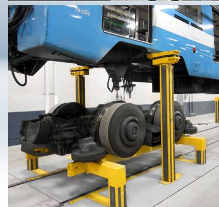
With underfloor lifting systems from Pfaff Verkehrstechnik, maintenance work can be comfortably performed on anything from trams to high-speed trains.
