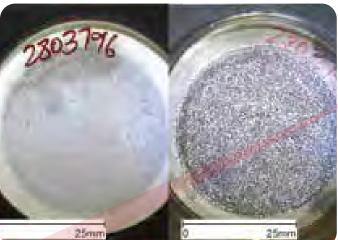
Sample of an unused grease that contains very finely-divided aluminium particles that act as a solid lubricant.
