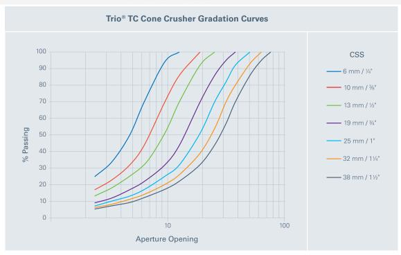
**NOTE:** the above graph relates to an application for medium hard rock, where the fines were removed and the feed contained no clay or moisture.
