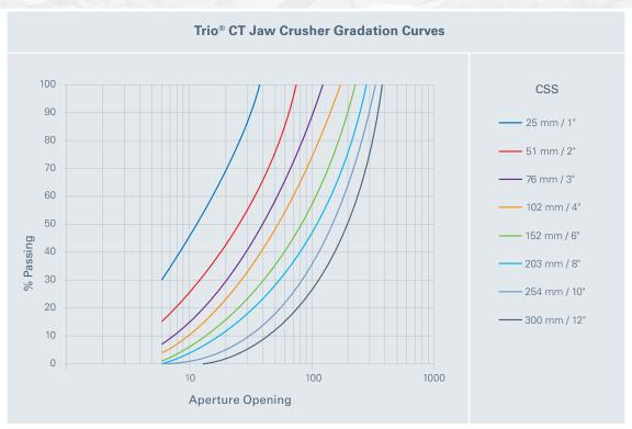
NOTE: the above graph relates to an application for medium hard rock, where the fines were removed and the feed contained no clay or moisture.
