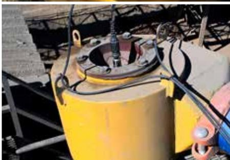
**Top:** Control and monitoring system sensor connected to the air core booster of a Cavex® hydrocyclone.
